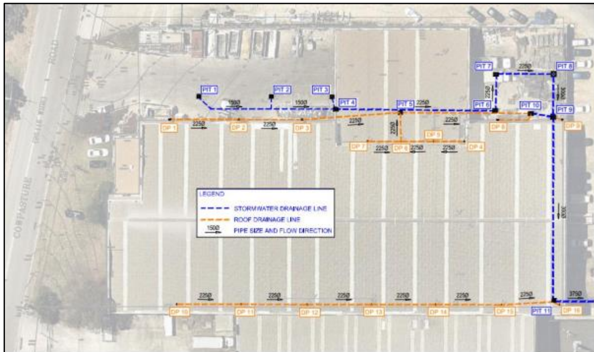
Figure 20: Existing stormwater network
